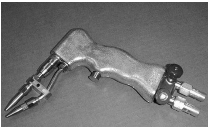
FIG. 15 The DHC 2000 Torch shown assembled for cutting sheet steel using the under cutter.
